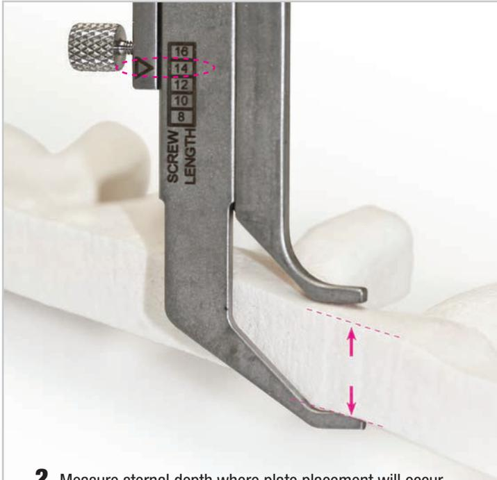
**2.** Measure sternal depth where plate placement will occur. Measure 3 points (manubrium, the lateral incision, and body). The measuring device indicates that a 14mm screw length would be recommended for plate placement (indicated by the arrows). The measuring device accounts for the thickness of the plate, so a 14mm screw would be used in this example.
